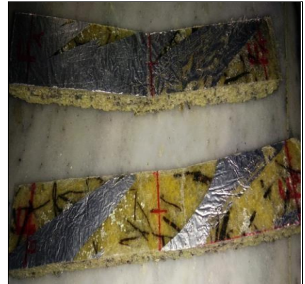
(c) Fractured specimen on Flexural Test
