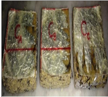
(b) Fractured specimen on Compression test
