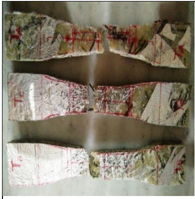
(a) Fractured specimen on Tensile test
